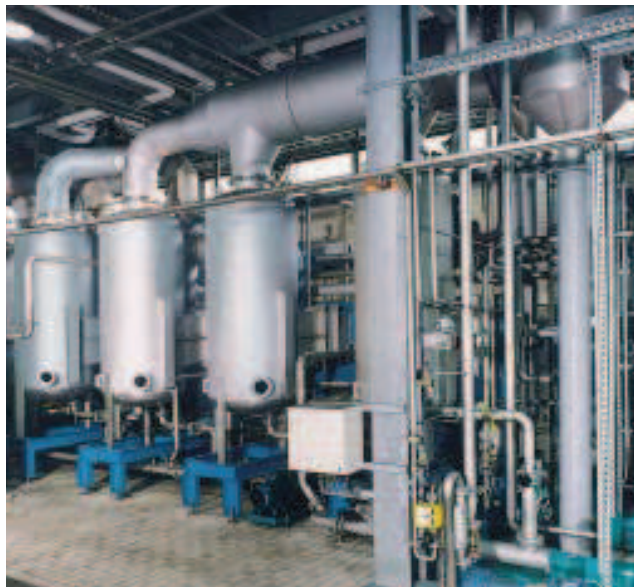
Multiple-effect plate evaporation plant for fructose. Evaporation rate: 16 t/hr
